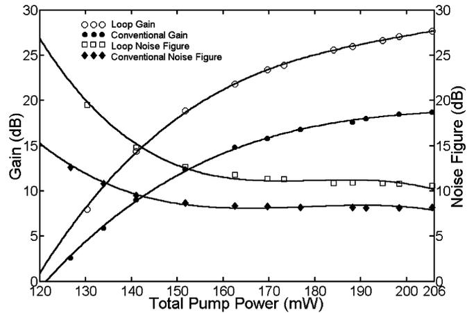
Fig. 3. Gain and NF variations as a function of total pump power for conventional and loop *L*-EDFA configurations. ( $P_{\text{sig.in}} = -30$  dBm,  $\lambda_{\text{sig}} = 1585$  nm).
