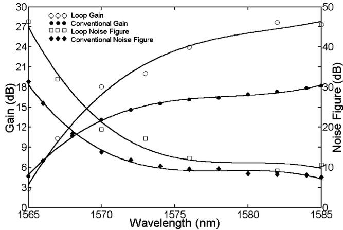
Fig. 4. Gain and NF variations as a function of signal wavelength for conventional and loop  $L$ -EDFA configurations. ( $P_{\text{sig,in}} = -30$  dBm,  $P_{\text{p,tot}} = 205.6$  mW).
