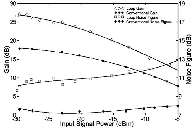
Fig. 5. Gain and NF variations as a function of input signal power for conventional and loop  $L$ -EDFA configurations. ( $\lambda_{\text{sig}} = 1585$  nm,  $P_{\text{p,tot}} = 205.6$  mW).
