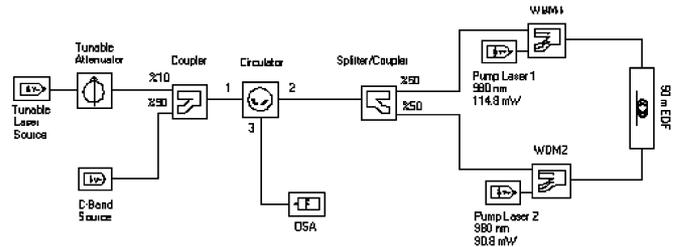
Fig. 1. *L*-band loop EDFA.
