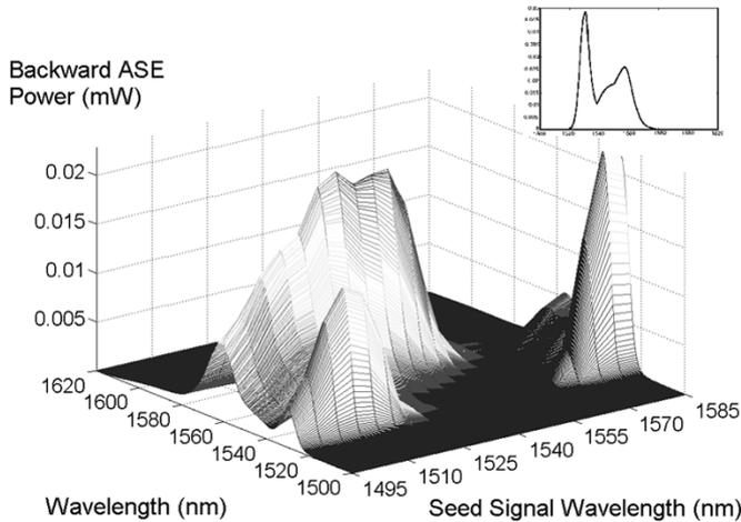
Fig. 2. Backward ASE spectrum of forward pumped *L*-EDFA as a function of seed signal wavelength. Inset: Backward ASE spectrum without seed signal.
