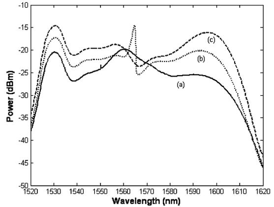
Fig. 4. Measured output spectra for different configurations (a) *C* + *L*-band loop ASE source with a seed signal power of  $-8$  dBm. (b) Conventional double-pass ASE source with a *C*-band FBG reflector. (c) Conventional double-pass ASE source with a fiber reflector and optimized reflection.
