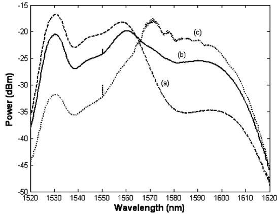
Fig. 3. Band selected output spectra of the loop ASE source for different seed signal powers (a) *C*-band without seed signal, (b) *C* + *L*-band with a seed signal power of  $-8$  dBm, and (c) *L*-band with a seed signal power of  $0$  dBm.
