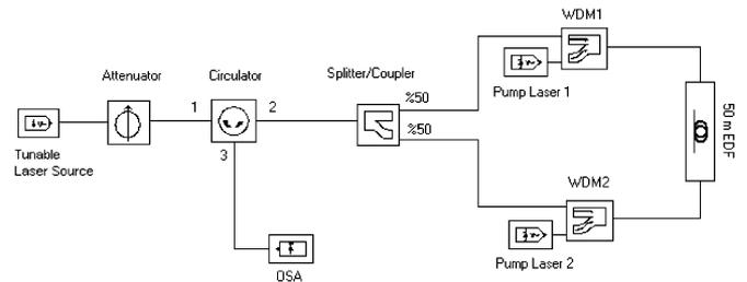
Fig. 1. Band selectable broadband loop ASE source.
