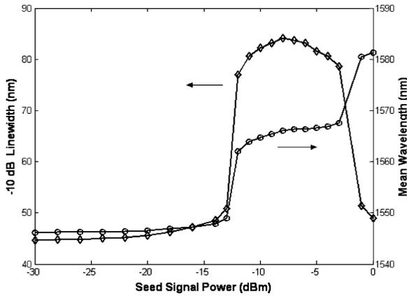
Fig. 5. The  $-10$ -dB linewidth and mean wavelength of the loop ASE source as a function of the seed signal power. ( $P_{p,tot} = 230.6$  mW).
