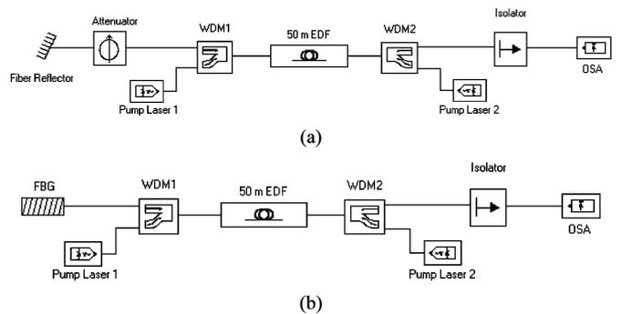
Fig. 2. Conventional bidirectionally pumped double-pass ASE source design with (a) gold-coated broadband fiber reflector and (b)  $C$ -band FBG reflector.
