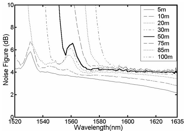
Figure 2. Noise figure spectrum of bidirectionally pumped EDFA with different fiber lengths. Total pump power =  $2 \times 150$  mW, Signal input power =  $-30$  dBm X 100 channels.
