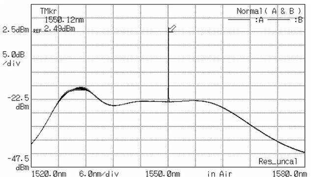
Figure 8. Output spectrum of C band EDFA.  $P_{pump\ in} = 92.5\ mW$  and  $P_{sig\ in} = -30\ dBm$ .
