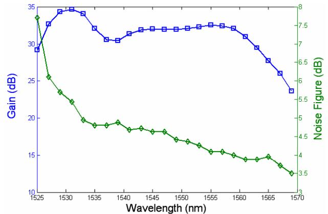
Figure 7. Gain and noise figure spectra of a 6 m long C band EDFA.  $P_{pump\ in} = 92.5\ mW$  and  $P_{sig\ in} = -30\ dBm$ .
