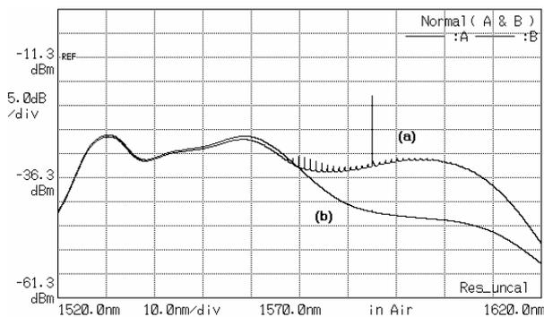
Figure 9. The output spectrum of bidirectionally pumped L band EDFA.  $P_{pump\ tot} = 205\ mW$  and  $P_{sig\ in} = -30\ dBm$ . (a) with the seed signal (b) without the seed signal.
