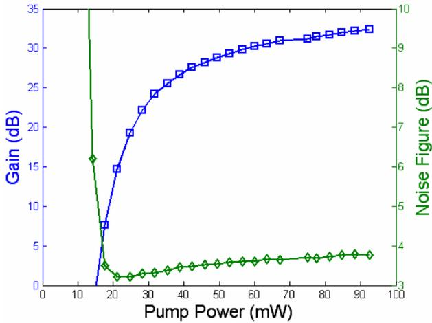
Figure 5. Gain and noise figure characteristics of a 6 m long C band EDFA as a function of pump power.  $P_{sig\ in} = -30\ dBm$ , Signal wavelength = 1550 nm.
