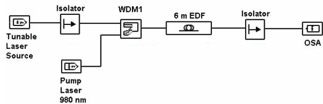
Figure 3. Forward pumped C band EDFA.
