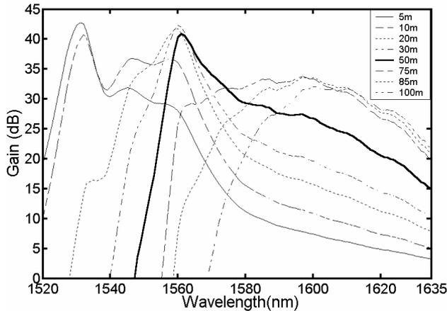
Figure 1. Gain spectrum of bidirectionally pumped EDFA with different fiber lengths. Total pump power =  $2 \times 150$  mW, Signal input power =  $-30$  dBm X 100 channels.
