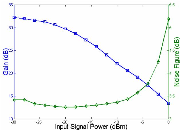
Figure 6. Gain and noise figure characteristics of a 6 m long C band EDFA as a function of input signal power.  $P_{pump\ in} = 92.5\ mW$ , Signal wavelength = 1550 nm.
