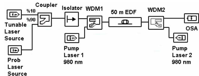
Figure 4. Bidirectionally pumped L band EDFA.
