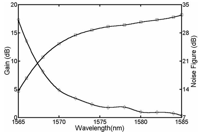
Figure 10. Gain and noise figure spectra of a 50 m long L band EDFA.  $P_{pump\ tot} = 205\ mW$  and  $P_{sig\ in} = -30\ dBm$ .
