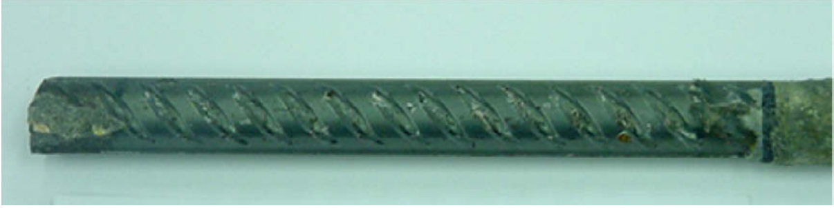
Fig. 2. Steel bar extracted from the concrete specimen contaminated with 2% chloride and incorporating CI-1 inhibitor [17].
