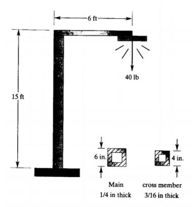
The lamp frame shown in the accompanying figure has hollow square cross sections and is made of steel, with  $E = 29 \times 10^6$  lb/in<sup>2</sup>. Using hand calculations, determine the endpoint deflection of the cross member where the lamp is attached.
