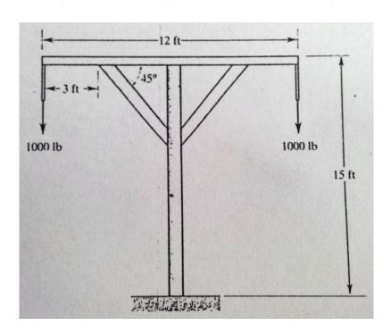
The frame shown in the accompanying figure is used to support a load of 2000 lb. The main vertical section of the frame has an annular cross section with an area of 8.63 in<sup>2</sup> and a polar radius of gyration of 2.75 in. The outer diameter of the main tubular section is 6 in. All other members also have annular cross sections with respective areas of 2.24 in<sup>2</sup> and polar radii of
