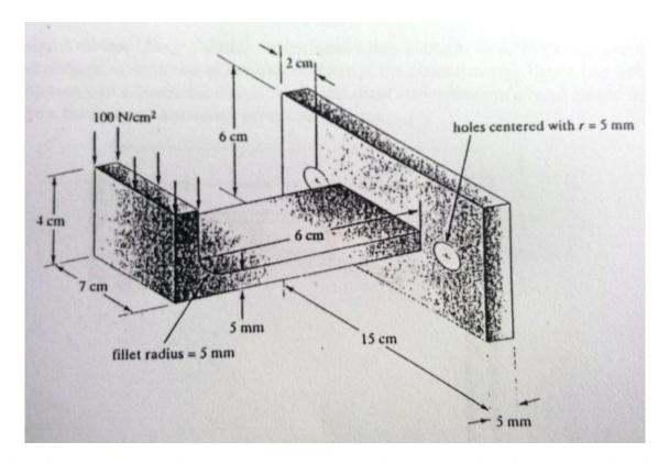
Using ANSYS, calculate and plot the principal stress distributions in the support component shown in the accompanying figure. The bracket is made of steel. It is fixed around the hole surfaces.
