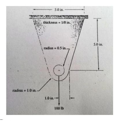
A  $\frac{1}{8}$ -in-thick plate supports a load of 100 lb, as shown in the accompanying figure. The plate is made of steel, with  $E=29\times 10^6$  lb/in<sup>2</sup> and  $\nu=0.3$ . Using ANSYS, determine the principal stresses in the plate. When modeling, distribute the load over part of the bottom portion of the hole.
