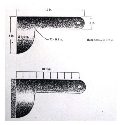
Consider one of the many steel brackets ( $E = 29 \times 10^6$  lb/in<sup>2</sup>,  $\nu = 0.3$ ) used to support bookshelves. The dimensions of the bracket are shown in Figure 6.33. The bracket is loaded uniformly along its top surface, and it is fixed along its left edge. Under the given loading and the constraints, plot the deformed shape; also determine the principal stresses and the von Mises stresses in the bracket.
