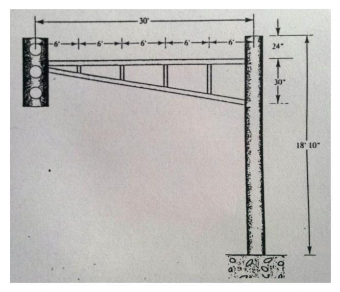
**Design Problem** Using a three-dimensional beam element in ANSYS, you are to size the cross sections of members of the frame shown in the accompanying figure. Use hollow tubes. The frame is to support the weight of a traffic light and withstand a wind gust of 80 miles/hr. Write a brief report discussing your final design.
