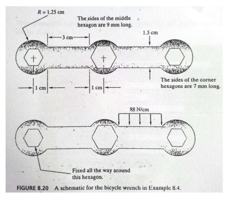
The bicycle wrench shown in Figure 8.20 is made of steel with a modulus of elasticity E = 200 GPa and a Poisson's ratio  $\nu = 0.32$ . The wrench is 3 mm thick. Determine the von Mises stresses under the given distributed load and boundary conditions.
