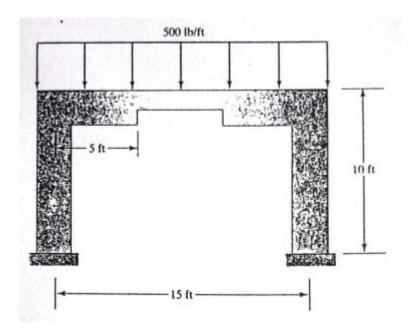
The frame shown in the accompanying figure is used to support a load of 500 lb/ft. Using ANSYS, size the cross sections of each member if standard-size steel square tubing is to be used. Use three different sizes. The deflection of the centerpoint is to be kept under 0.05 in.
