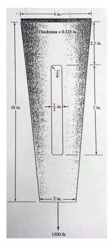
Consider a plate with a variable cross section supporting a load of 1500 lb, as shown in the accompanying figure. Using ANSYS, determine the deflection and the x- and y-components of the stress distribution in the plate. The plate is made of a material with a modulus of elasticity  $E = 10.6 \times 10^3$  ksi. In Problem 24 of Chapter 1, you were asked to analyze this problem using simple direct formulation. Compare the results of your direct-formulation model
