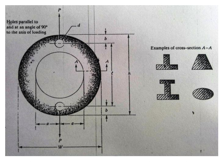
**Design Problem** Referring to one of the design problems in Chapter 8 (Problem 22), each student is to design and construct a structural model from a  $\frac{3}{8}$ "  $\times$  6"  $\times$  6" sheet of plexiglas material that adheres to the specifications and rules given in Problem 22. Additionally, for this project, the model may have any cross-sectional shape. Examples of some common sections are shown in the accompanying figure.
