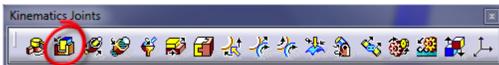
Figure 55 – Kinematics Joints toolbar with Prismatic Joint selected
