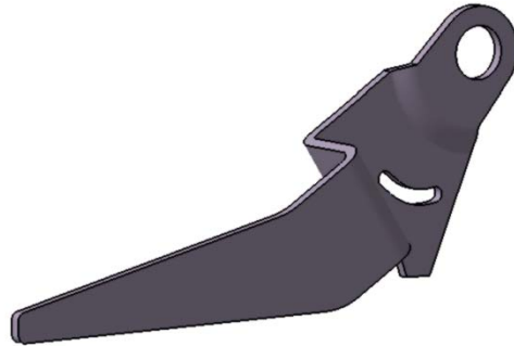
Figure 16 – Backrest Lever 3D-CAD model
