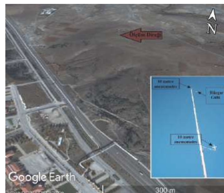
Wind Measurement Station (10 m and 30 m)
