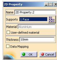
2D Property provides thickness and material
